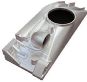
Main Image: A five-piece weldment part that MAC Machine produces is difficult to machine because of the complex geometries of the unit.
